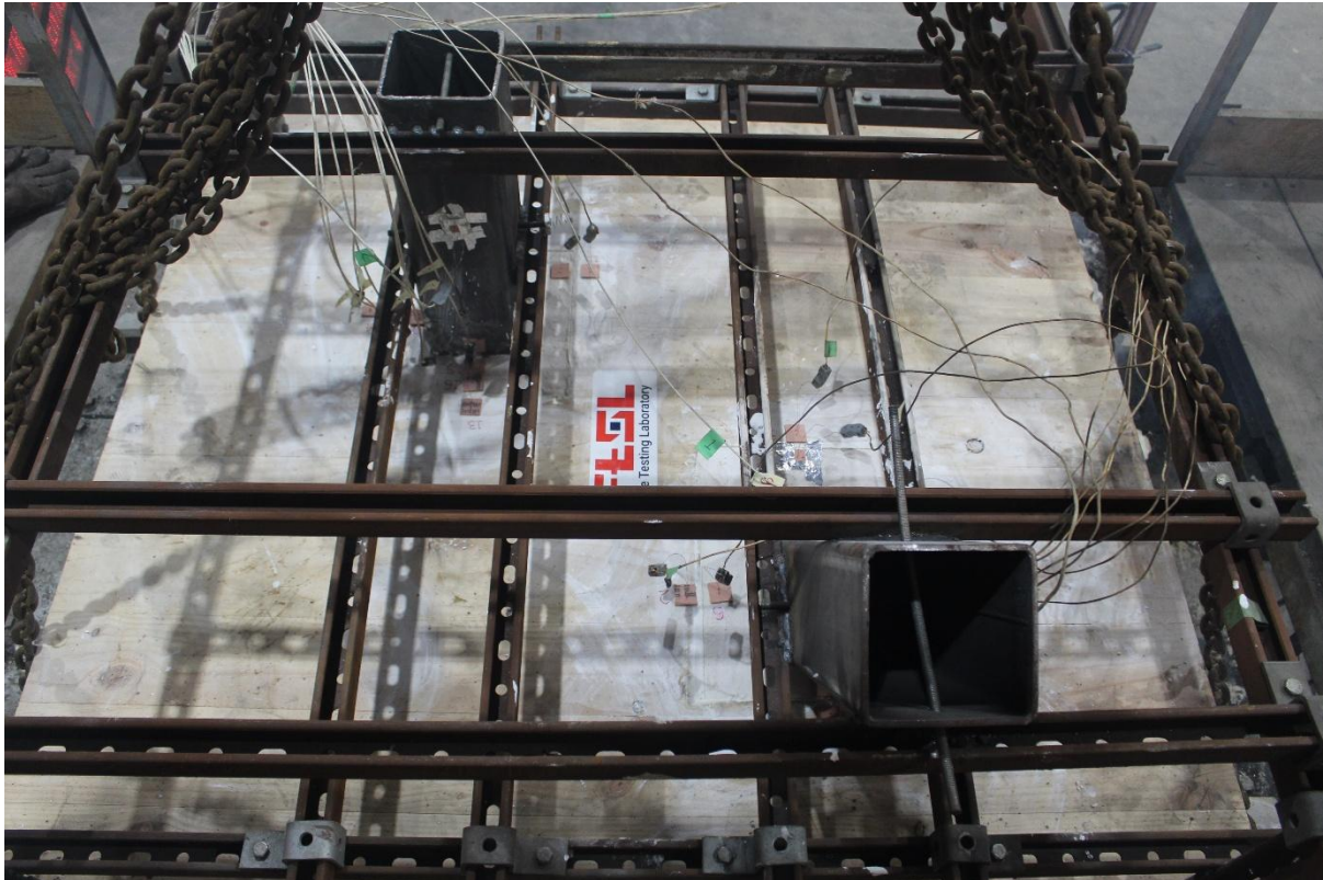
Figure 12 - Unexposed face at 45 minutes
