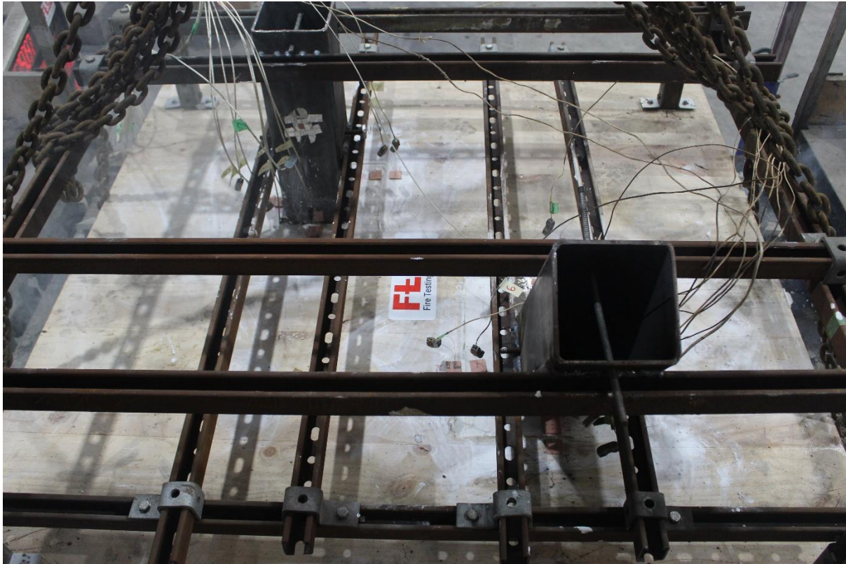
Figure 8 - Unexposed face at 15 minutes
