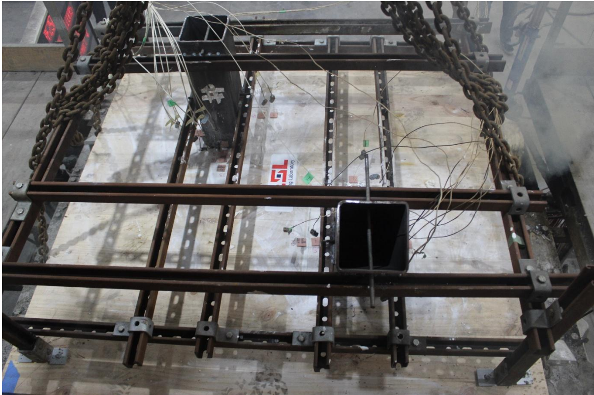
Figure 16 - Unexposed face at 90 minutes
