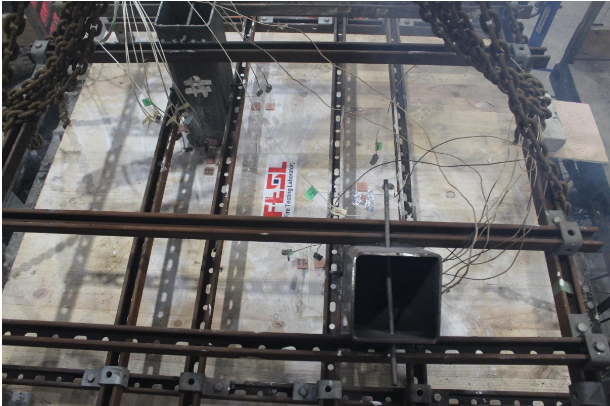
Figure 14 - Unexposed face at 60 minutes
